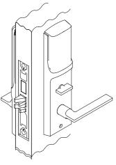
Note: Strike & dust box@ are used on door frame. Both outside and inside leaver sets should be cleaned up by soft and dry cloth to keep it shining. It is strictly forbidden to use organic solution and corrosive chemicals on the surface.
