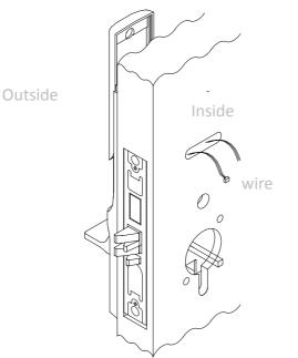
5. Install cylinder clockwise and tighten the cylinder screws on the side. Checking function by turning the key back and force.
